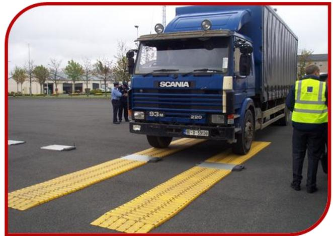
*Above: Axle weighers can be used to ensure compliance*
