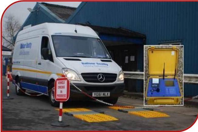
VOSA has been investing in technology to pinpoint non-compliant vehicles much more precisely. VOSA uses a combination of high-speed in-motion weighing, automatic number plate recognition and the Operator Compliance Risk Score (OCRS) system to decide which vehicles should be inspected.
